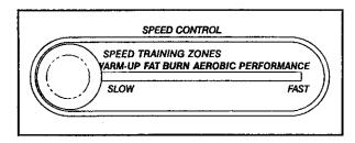
Next, slowly slide the speed control to the right until the walking belt begins to move at slow speed. Carefully step onto the walking belt and begin exercising. Change the speed of the walking belt as desired by sliding the speed control.
